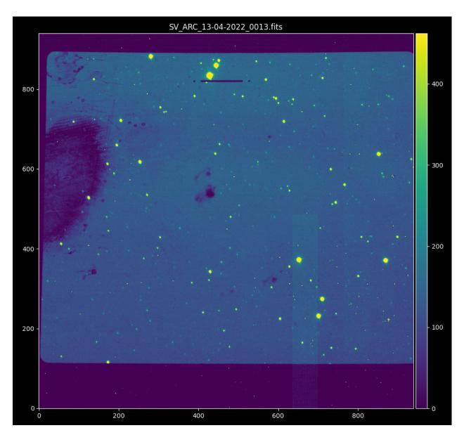
The slit is visible near the top center.
