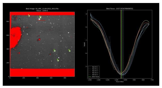
The sources used are plotted to the left and to the right you get the data and fitted models plot. The dashed vertical lines represent the best focus for each individual star. The solid vertical line represent the best focus value.
