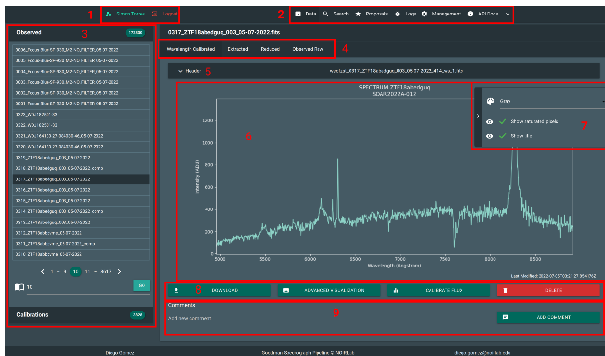
Fig. 3: Detail: 1. Access to user controls and information. 2. Main navigation bar. 3. Quick access to files. 4. Related or child files. 5. Toggle header view. 6. Visualization area. 7. Visualization options. 8. Contextual actions. 9. Comments.
